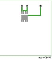
Fig. 6. PCB layout for thermal resistance junction to ambient minimum footprint; FR4 Board; 2oz copper
