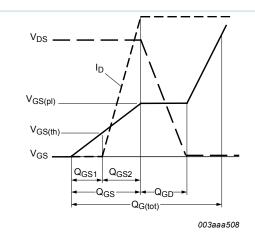
Fig. 15. Gate charge waveform definitions
