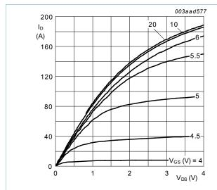
Fig. 5. Output characteristics: drain current as a function of drain-source voltage; typical values  $T_{J}=25\,^{\circ}C$
