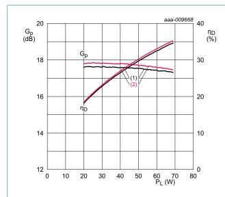
$V_{DS}$  = 28 V;  $I_{Dq}$  = 1600 mA; carrier spacing = 5 MHz;  $\delta$  = 46 %.
