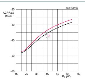
$V_{DS}$  = 28 V;  $I_{Dq}$  = 1600 mA; carrier spacing = 5 MHz;  $\delta$  = 46 %.
