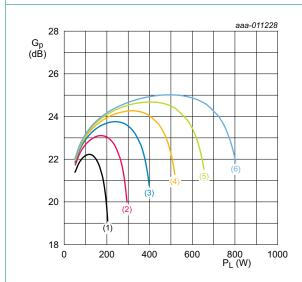
$I_{Dq} = 100 \text{ mA}$ ; f = 108 MHz;  $t_p = 100 \text{ } \mu\text{s}$ ;  $\delta = 20 \text{ } \%$ .
