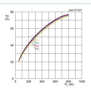
$V_{DS}$  = 50 V; f = 108 MHz;  $t_p$  = 100  $\mu$ s;  $\delta$  = 20 %.
