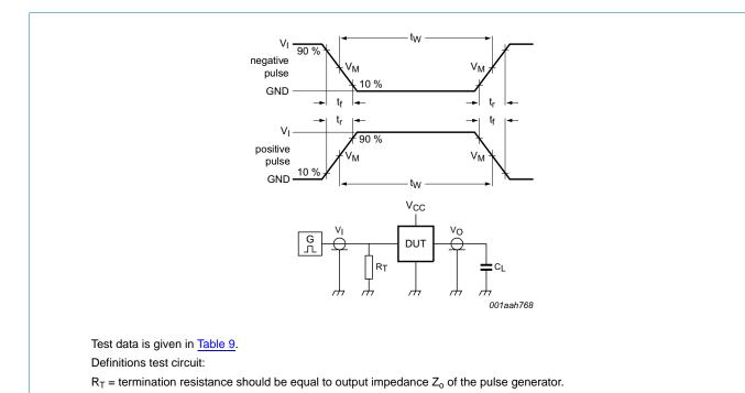
$C_L = \mbox{load capacitance including jig and probe capacitance}. \\$  Fig 8. Test circuit for measuring switching times
