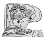
3. Insert the memory card into the memory card slot as shown in the diagram below:
