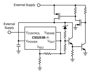
Figure 21. This Circuit Is an Example of How the CS5253B-1 Can Be Short-Circuit Protected When Operating With V<sub>OUT</sub> > 6.0 V
