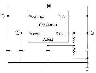
Figure 22. Diode Protection Circuit
