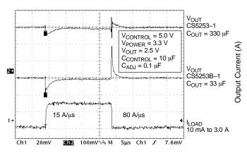
Figure 5. Transient Response Comparison between CS5253-1 and CS5253B-1
