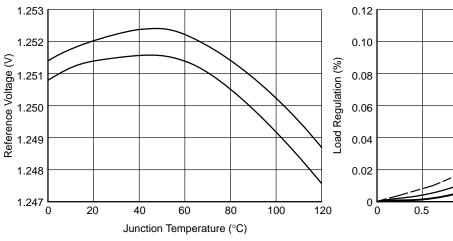
Figure 3. Reference Voltage vs Junction Temperature
