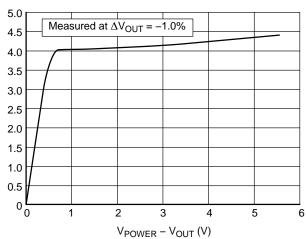
Figure 6. Output Current vs  $V_{POWER} - V_{OUT}$
