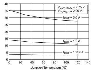
Figure 16. V<sub>CONTROL</sub> Supply Current vs Junction Temperature
