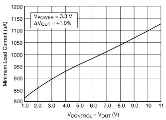
Figure 8. Minimum Load Current vs V<sub>CONTROL</sub> - V<sub>OUT</sub>
