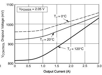
Figure 11. V<sub>CONTROL</sub> Only Output Current vs Junction Temperature
