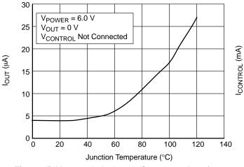
Figure 15. V<sub>POWER</sub> Only Output Current vs Junction Temperature
