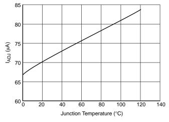
Figure 7. Adjust Pin Current vs Junction Temperature
