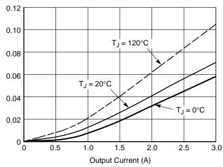
Figure 4. Load Regulation vs Output Current
