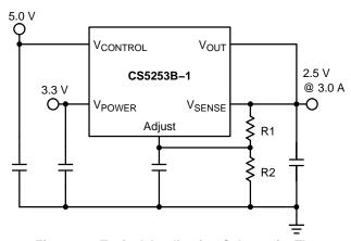
Figure 20. Typical Application Schematic. The Resistor Divider Sets V<sub>OUT</sub>, With the Internal 1.260 V Reference Dropped Across R1.
