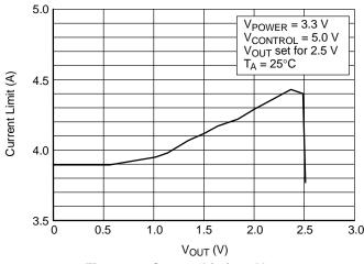
Figure 17. Current Limit vs VOUT
