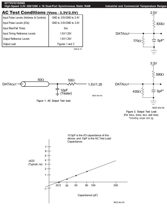
Figure 3. Typical Output Derating (Lumped Capacitive Load).
