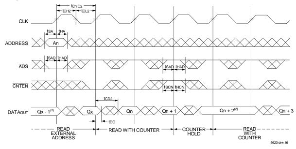
Timing Waveform of Flow-Through Read with Address Counter Advance<sup>(1)</sup>
