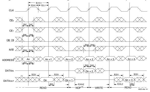
Timing Waveform of Flow-Through Read-to-Write-to-Read ( $\overline{OE}$  Controlled)<sup>(2)</sup>
