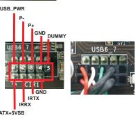
Step3. Install Multi-Angle CIR Receiver to the front USB port. If Multi-Angle CIR Receiver cannot successfully receive the infrared signals from MCE Remote Controller, please try to install it to the other front USB port.
