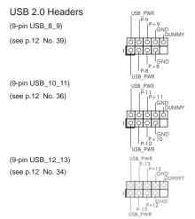
Besides six default USB 2.0 ports on the I/O panel, there are three USB 2.0 headers on this motherboard. Each USB 2.0 header can support two USB 2.0 ports.
