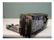
Step2. If required, connect the auxiliary power source to the PCI Express graphics cards.
