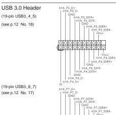
Besides two default USB 3.0 ports on the I/O panel, there are two USB 3.0 headers on this motherboard. Each USB 3.0 header can support two USB 3.0 ports.
