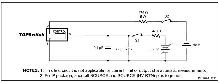
Figure 14. TOPSwitch General Test Circuit.
