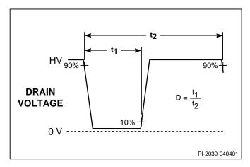
Figure 10. TOPSwitch Duty Cycle Measurement.
