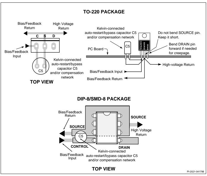
Figure 9. Recommended TOPSwitch Layout.
