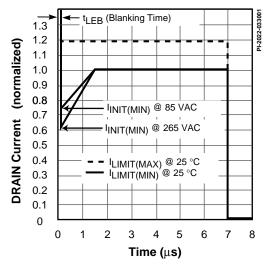
Figure 12. Self-protection Current Limit Envelope.
