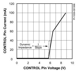
Figure 11. TOPSwitch CONTROL Pin I-V Characteristic.
