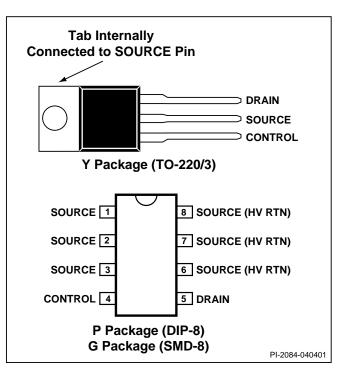
Figure 3. Pin Configuration.
