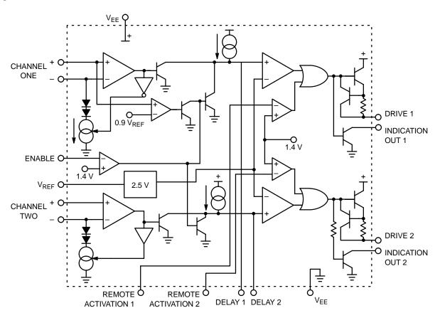
Figure 17. MC3424/MC3524 Equivalent Circuit
