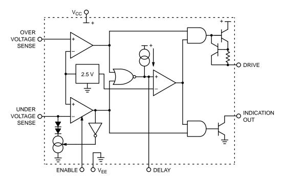
Figure 18. MC3425/MC3525 Equivalent Circuit
