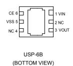
\* The dissipation pad for the USP-6B package should be solder-plated in recommended mount pattern and metal masking so as to enhance mounting strength and hear release. If the pad needs to be connected to other pins, it should be connected to the VSS pin.
