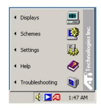
**Settings** - This option lets you configure the ATI IGP Catalyst<sup>™</sup>, advanced display settings, and device settings. This menu also allows you to restore the default display settings.
