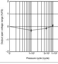
Even after testing for 1 million times, the variations in the offset voltage and output span voltage are minimal.
