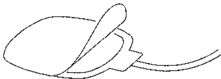
Figure 5-2 Peeling the Liner from the Electrode
