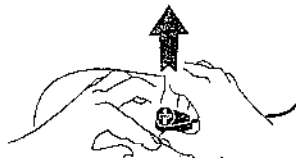
Figure 5-6 Disconnecting Defibrillation Cable from FAST-PATCH Electrodes
