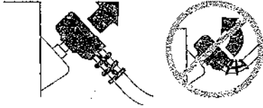
Figure 5-7 Disconnecting Defibrillation Cable from Test Post
