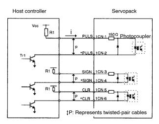
Note The signal logic for open collector output is as follows.
