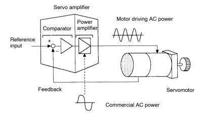
A servo amplifier consists of the following two sections:
