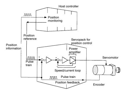
The host controller can send a position reference (pulse train) to the Servopack to perform positioning or interpolation.
