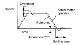
In other words, the mode switch is a function that automatically switches the speed control mode inside the Servopack from PI control to P control while certain conditions are being established.
