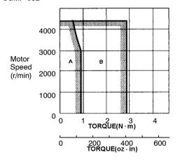
A: Continuous Duty Zone B: Intermittent Duty Zone 5.2.2 Mechanical Characteristics
