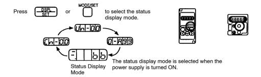
Keys to the status display are shown below. Note that the display differs between the speed/torque control (SGDA - $\square\square\square$ S) and position control (SGDA - $\square\square\square$ P) types.
