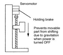
NOTE The built-in brake in Servomotor with brake is a de-energization operation type, which is used for holding purposes only and cannot be used for braking purposes. Use the holding brake only to retain a stopped motor. Brake torque is more than 100% of the rated motor torque.
