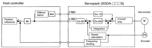
KP: Position loop gain KFF: Feed-forward gain
