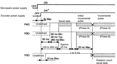
\*Encoder power is automatically turned ON inside the Servopack.
