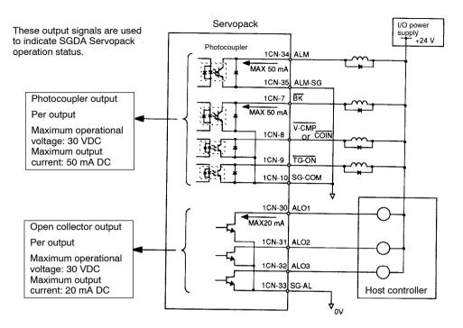
Note Provide an external I/O power supply separately.
