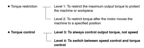
This section describes how to use levels 3 and 4 of the torque control function.
