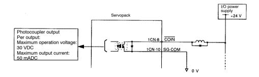
3.7.3 Using Positioning Complete Signal cont.
