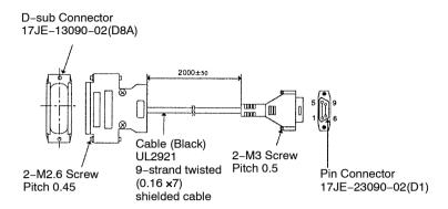
Note: Fold back the cable shielding at each end of the cable and secure it with clamp.
