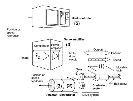
(1) Controlled system: Mechanical system for which the position or speed is to be con-
