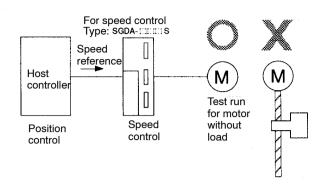
**NOTE** Check the motor operation with the motor disconnected from the machine. If the host controller does not perform position control correctly, the motor may run out of control.
