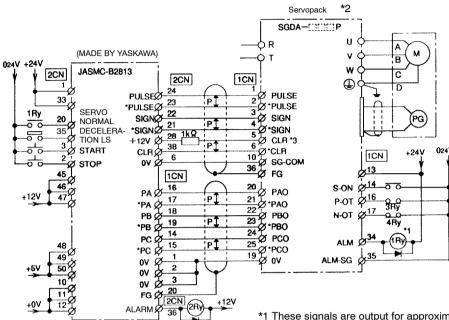
\*1 These signals are output for approximately two seconds when the power is turned ON. Take this into consideration when designing a power ON sequence. Relay 1Ry is used to stop main circuit power supply to Servopack.
