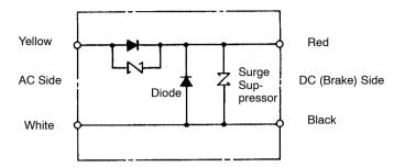
• Internal Circuit for 100 VAC Input (LPDE-1H01)
