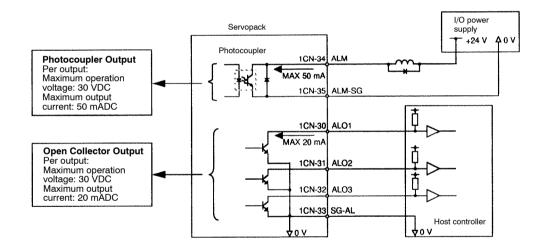
Provide an external I/O power supply separately. There are no DC power available from Servopack for output signals.
