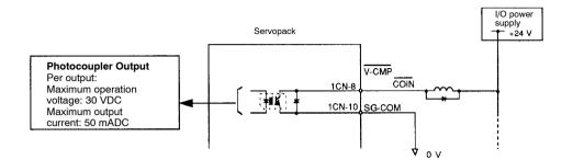
Output → V-CMP 1CN-8 Speed Coincidence Output For Speed/Torque Control Only
