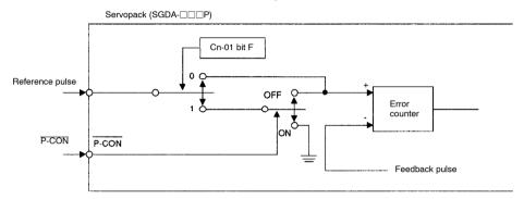
Note: Whether INHIBIT function is used, select by bit F of Cn-01.
