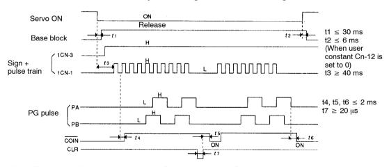
Note The interval from the time the servo ON signal is turned ON until a reference pulse is input must be at least 40 ms. Otherwise, the reference pulse may not be input. The error counter clear (CLR) signal must be ON for at least 20 μs. Otherwise, it becomes invalid.
