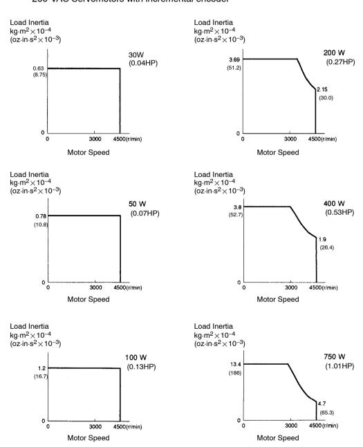
**Note** The above diagrams represent deceleration under maximum torque. Applying an acceleration/deceleration curve to the reference allows operation outside the range of the diagrams. (That is, characteristics change according to pattern of operation and load conditions).
