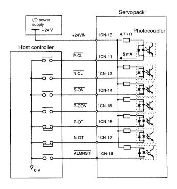
Note Provide an external I/O power supply separately.
