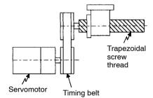
To develop an excellent servo system, it is important to select a rigid drive system that has no play.
