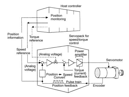
Set the user constants for Servopack to switch between the following torque control modes:
