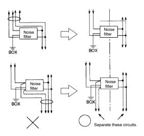
• Separate the noise filter ground wire from the output lines.
