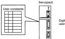
Digital Operator is used to set user constants.
