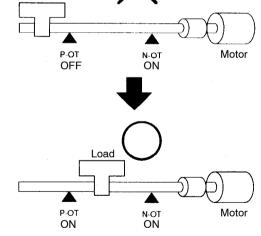
Conduct autotuning when no overtravel has occurred (both P-OT and N-OT signal ON).
