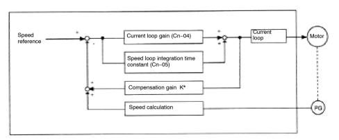
\* Compensation gain (K) is in proportion to the compensation constant (user constant Cn–28). Cn–28 = 0 shows no compensation status.
