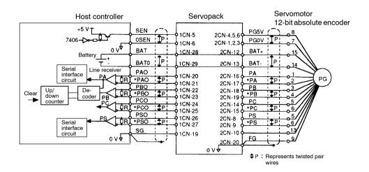
Line Receiver Used: SN75175 or MC3486 manufactured by Texas Instruments Inc. Termination Resistor R: 220 to 470  $\Omega$
