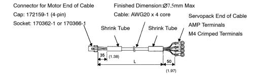
b) Cables For Motor With Brake (with connector and AMP terminals)
