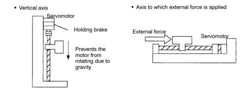
NOTE To prevent faulty operation caused by gravity (or external force), first check that the motor and holding brake operate normally with the motor disconnected from the machine. Then, connect the motor to the machine and conduct a test run.
