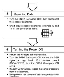
NOTE Setting up the encoder sets the revolution count inside the encoder to 0.
