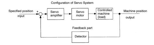
This servo system is an automatic control system that detects the machine position (output data), feeds back the data to the input side, compares it with the specified position (input data), and moves the machine by the difference between the compared data.
