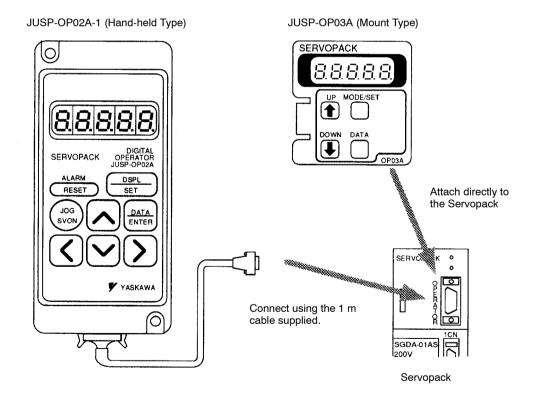
• The Digital Operator connector can be connected or disconnected while the Servopack power is ON.
