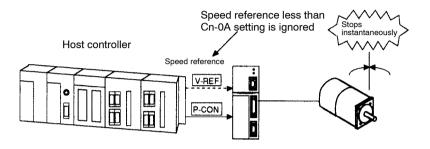
2) Set the following memory switch so that input signal P-CON can be used to enable or disable the zero-clamp function.
