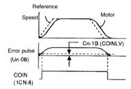
Set the number of error pulses in terms of reference unit (the number of input pulses that is defined using the electronic gear function).
