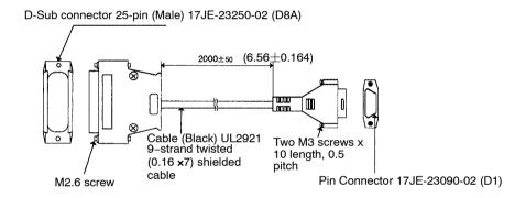
Note: Fold back the cable shielding at each end of the cable and secure it with clamps.
