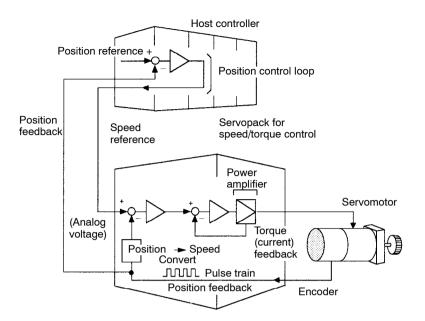
As shown in the figure above, a position control loop is formed in the host controller. The host controller compares a position reference with a position feedback signal and sends processing results to the Servopack as a speed reference.
