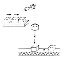
• Overhanging Load Example 2: Tension control drive
