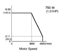
**Note** Diagrams above represent deceleration under maximum torque. Applying an acceleration/ deceleration curve to the reference allows operation outside the range of the diagrams. (That is, the characteristics change according to pattern of operation and load conditions).
