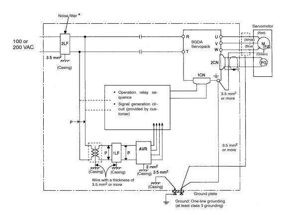
c) The following is an example of wiring for noise control.
