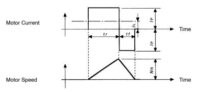
Motor Current (size) - Motor Speed Timing Chart
