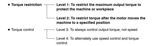
This section describes how to use levels 1 and 2 of the torque restriction function.
