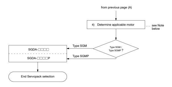
Note The applicable motor type (SGM/SGMP) can be changed by setting the user constants.
