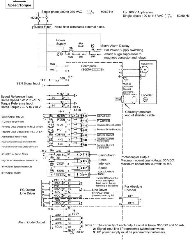
6.2.3 Internal Connection Diagram and Instrument Connection Examples cont.
