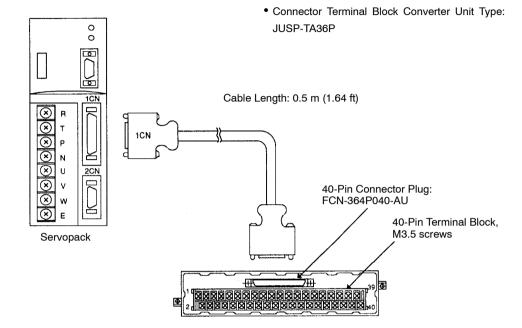
2) The relationships between terminal block pin numbers and signal names are shown in the table below.
