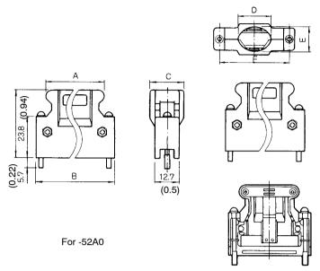
Diagram of Assembled Connector (for reference)
