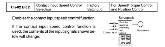
When this memory switch is reset, the meanings of the following signals will also change:
