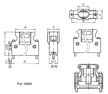
Diagram of Assembled Connector (for reference)
