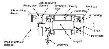
Yaskawa SGM and SGMP Servomotors are of the synchronous type.
