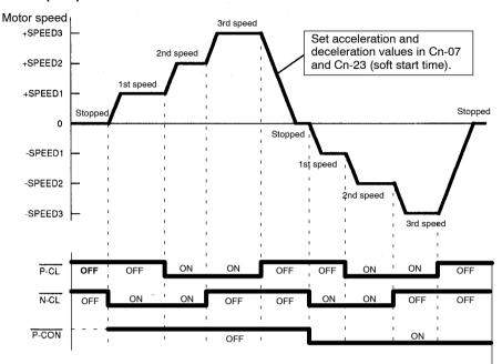
**Note** For the position control type, the soft start function is available only when contact input speed control is used. The soft start function is not available when pulse reference input is used.
