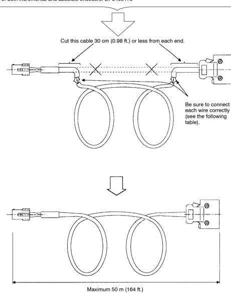
2) Connect cables of the same color to each other as shown in the table below. Note that wiring for incremental and absolute encoders is different.
