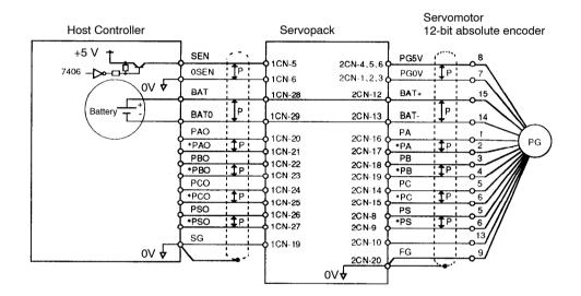
The battery voltage is not internally monitored in the Servopack. Therefore, detect low battery voltage at the host controller.
