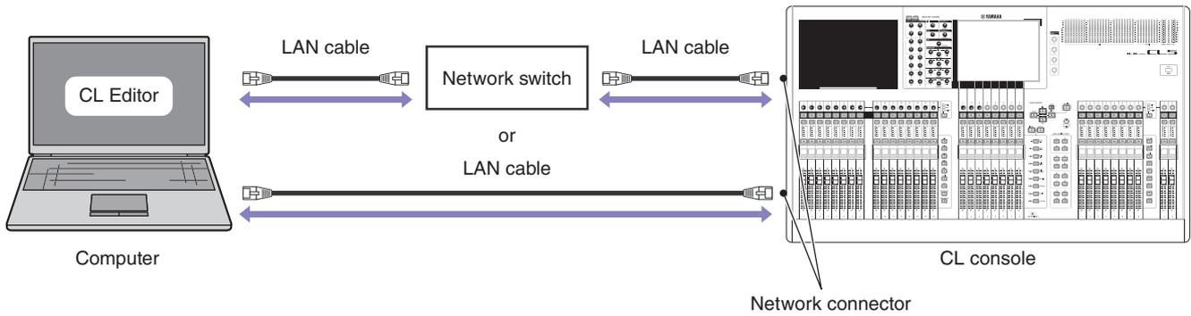
**NOTE** You cannot simultaneously control one CL unit from two computers running CL Editor. However, you can control the CL unit using CL Editor on a computer along with the CL StageMix application installed on an iPad (or iPad2) that is connected via WiFi.
