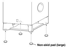
Attach the non-skid pads (large) to the bottom of the subwoofer, and then place the subwoofer on a level hard floor.
