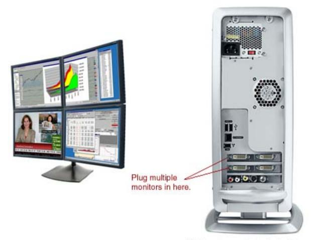
Picture shows dual output video cards, PC configurations may vary.
