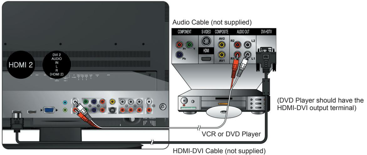
**4. Connecting to External Stereo System to Listen to LCD TV Sound**
