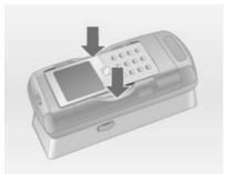
With side brackets of the adapter opened, vertically lower the mobile phone into the adapter as shown in the above figure until the side brackets snap in.
