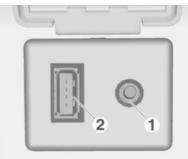
In the centre console there is a USB socket **2** for the connection of external audio sources.
