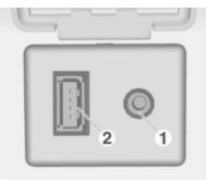
In the centre console there is an AUX socket **1** for the connection of external audio sources.
