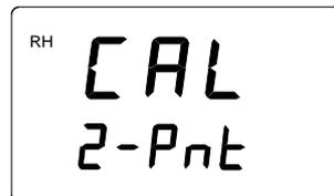
Press **ENTER** and the following text appears on the display for about 1 ... 2 seconds:
