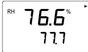
Numbers on the first line indicate the RH measured by the transmitter, and numbers on the second line indicate the RH measured by the HMI41 probe. Let the readings stabilize. Press **MODE**, and a text similar to the following appears:
