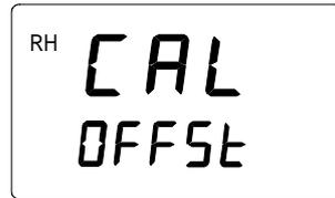
If you press the **HOLD** button, you will go on to two-point calibration mode, and if you press the **MODE** button, you will go on to gain calibration mode. You can return to offset calibration mode from two-point or gain calibration modes by pressing **MODE** or **HOLD** repeatedly. As offset and gain calibrations are performed in the same way, the following chapter is valid for both. For two-point calibration, see Two-Point Calibration on page 18.
