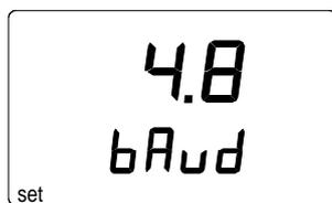
If the baud rate on the HMI41 display is not the same as that of the transmitter, change it with buttons ▲ and ▼. Use baud rate 19200 (= 19.2 on the HMI41 display) with the HMT100 and HMT330 series. When the baud rate is the same, press **ENTER** and the following appears:
