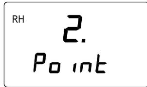
Insert the transmitter probe to the higher humidity. Within 1 ... 2 seconds, the display will automatically change to show a text similar to the following:
