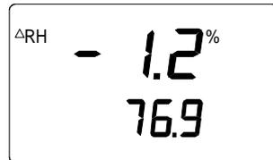
Numbers on the first line indicate how much the transmitter reading differs from that of the HMI41 reference probe. Numbers on the second line indicate the RH measured by the reference probe. You can return to the previous display by pressing **HOLD** again.
