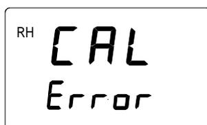
In this case, perform the calibration again. Whether the calibration was successful or not, HMI41 always returns to show the selected calibration mode:
