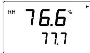
Numbers on the first line indicate the RH measured by the transmitter, and numbers on the second line indicate the RH measured by the reference probe. Let the readings stabilize. If you prefer, you can change the display to show the difference in the readings. Press **HOLD** and a text similar to the following appears:
