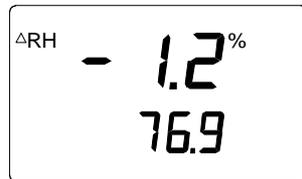
Numbers on the first line indicate how much the RH measured by transmitter differs from that of the reference probe. Numbers on the second line indicate the RH measured by the reference probe. If you wish, you can now calibrate the transmitter (by pressing MODE again the measured values appear on the display):
