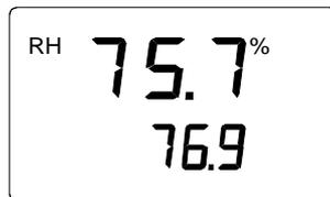
Numbers on the first line indicate the RH measured by the transmitter, and numbers on the second line indicate the RH measured by the HMI41 reference probe. If you wish, you can now adjust the transmitter:
