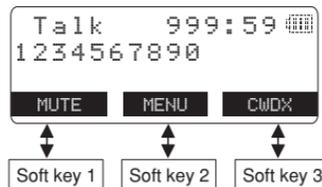
Soft key functions consists of soft key icons and soft keys (No. 1, 2, and 3). Each soft key corresponds to the icon displayed above, and each icon will be changed depending on the operation. Press the corresponding soft key to enter a menu, or select an item. In this manual, we refer to this combination of icons and keys as the soft key.
