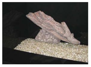
3. The rear right log has two holes on the base that insert over the studs at the back of the firebox (see photos below). Slide it to the left so it contacts the rear left log and the back wall of the firebox.
