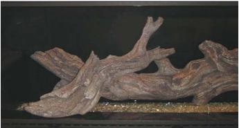
5. The front right log has a hole on the base that fits over the last pin on the firebox floor. Position the log as shown below with the front of the log resting on the ledge near the glass frame with approximately 2" gap to the glass opening.
