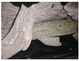
10. Replace the glass frame and start the fireplace. Let the fireplace burn for 30 minutes on high and check the logs for sooting. Remove the glass and carefully inspect the areas above the burner for soot accumulation. If any soot is detected, re-adjust the log and repeat this step to insure no sooting occurs.
