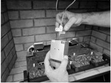
5. Loosen the lower 2 set screws holding the bulb in place until the bulb becomes loose.
