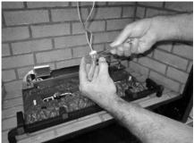
6. Replace the bulb and tighten the set screws (do not over-tighten, this will damage the bulb). (**NOTE**: .Take care to not touch the bulb with your fingers – use foam packing or paper towel to hold the bulb):
