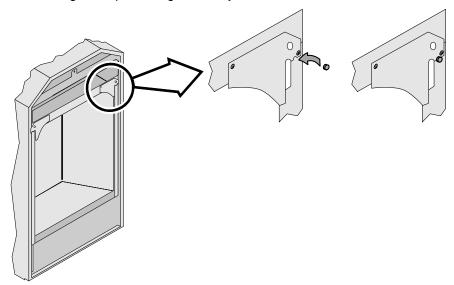
Position the face so the bottom brackets insert into the slots on the lower support legs (see "a" in the illustration below). With the brackets inserted, rotate the face forward until the magnets secure the face in place (see "b" below).
