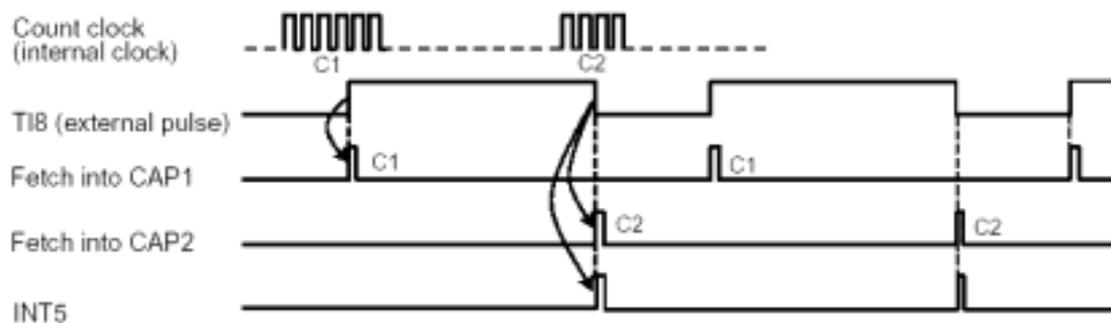
Figure 1 Measurement the high-level width
