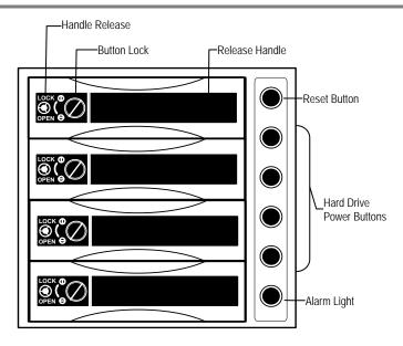
NOTE: The Alarm Light will turn on if the Hard Drives reach a temperature above safe operating conditions
