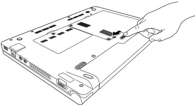
*(Sample Illustration) Locking the battery release lock*
