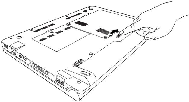
*(Sample Illustration) Unlocking the battery release lock*
