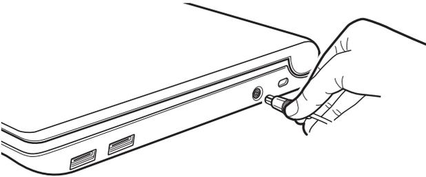
*(Sample Illustration) Connecting the AC adaptor cord to the computer*
