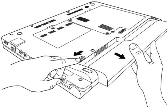
*(Sample Illustration) Removing the battery*
