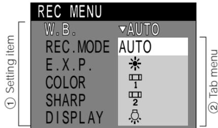
**4** Use the ▲ or ▼ buttons to select the desired setting from the tab menu ②, and press the ENTER button.
