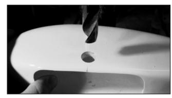
5.To install the wheel pants drill a hole that is big enough to go over the axle nut. Then you will need to install the wheel pants after you install the axels. The wheel pants are held on with 2-4-40 bolts and blind nuts. We recommend using a little bit of silicone between the landing gear and the wheel pant to help reduce vibration.
