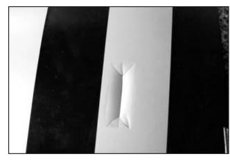
19. First thing is to cut the servo bay opening out. We decided to leave the covering in place and iron it down this will eliminate the covering from lifting or coming off in fight.
