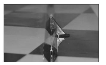
26. Attach the horns on the elevator control surface in the same manner
