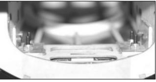
3. First cut the covering off the bottom of the plane where the four bolts and nylon lock nuts will be used to attach the landing gear.
