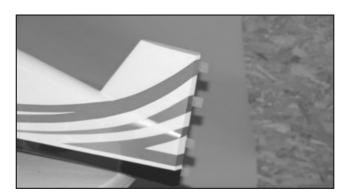
15. Allow them to dry and glue on the rudder. While the rudder is drying this is a good time to attach the tail gear.
