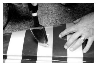
20.Use your iron to iron down the covering into the servo bay, some minor trimming of the covering may be necessary.
