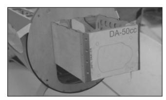
12. Once the glue is dry you can install the angle iron with nuts and bolts provided. You can also put on the engine template with a small amount of spray adhesive so it can be peeled of at a later time.
