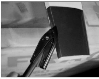
2.Use a heat gun and iron to go over all of the covering If bubbles show up you can use a small needle to puncture the bubble and then iron it down. On a multi layer area make sure to only puncture the top layer.
