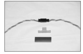
22.Next you will install the servos, the outboard servo will need a 6" extension installed on the servo wire. On our installation we used heat shrink to join the servo extension to the servo wire. We also used a plastic sleeving to go over the servo wires to protect them from chafing. See figures below.
