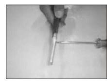
25. Once the four holes are drilled, install the metal arm to the wheel using the screws supplied with the kit.
