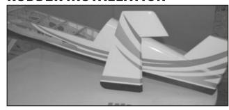
14.0il the hinge as you did for the aileron and glue hinge into the fuselage.
