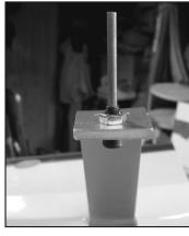
4.Install the wheel axels as shown. Make sure and use loc-tite and the threads.
