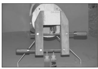
11. You will need to calculate the engine box length to determine the cowl length.Place the cowl on a level surface no place a straight edge. Across the top no measure from the bottom of the cowl to the straight edge. Now subtract a quarter inch from that measurement since the mount. Ring is a quarter inch inside the cowl. Now measure your engine. From the rear of the mounting plane to the surface that your prop will rest on.
