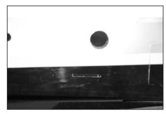
31.Locate the pull/pull exit holes located in the fuse. Use a sharp x-acto knife to cut the covering away from these exits.
