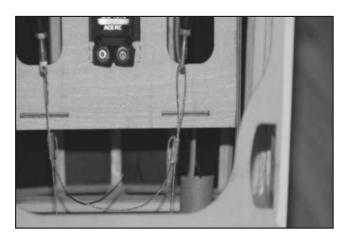
32.Complete the assembly as shown in the above picture. When crimping the cable with the brass tube that is included make sure you fish the cable through the crimp at least 2 times. After you crimp the brass tube use some thin C/A for a little extra security.
