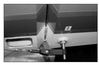
30. For the rudder control horn installation you will now drill the second hole to counter sink the head of the control horn. During installation you will need to make sure that the control horn is even on both ends.
