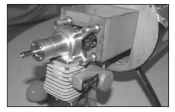
13. You cut out may vary depending on what engine you are using. Now is time to cut out for the carb. You can see we are mounting a DA 50. It is done with a rotary tool and a cutting bit. Now mark the center of your engine bolt holes with a ice pick or a spring loaded center punch. Also depending on what engine you use you may need standoff as in the picture below.
