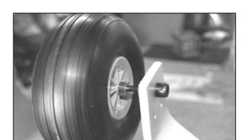
6.Install the tires included in the kit with the wheel collars that are supplied in the hardware package. Center the tire in the wheel pants and tighten down the wheel collars. Also once the wheel is centered in the wheel pant we suggest you grind a flat on the axel to prevent collar movement. Don't forget to put loc-tite on the wheel collar set screws.
