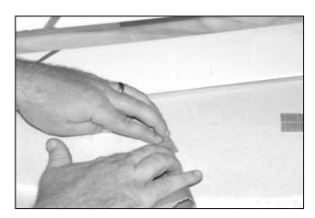
8.Sand the hinges so the glue will adhere well.Next glue the hinge to the wing side and allow the glue to dry. Repeat the process on the aileron now.
