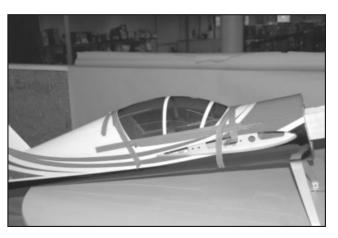
20. Attach the hatch to the fuse with screws provided this will allow the best fit of the canopy to the hatch.
