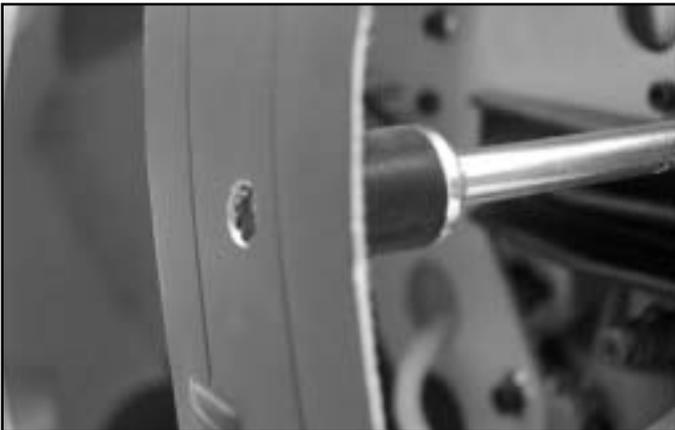
**23.** Install the big Damper in place as shown then drill 3/8" (9mm) hole. Never drill the hole on the molded mark as it is only for reference, please drill the hole and aim to the damper screw hole.
