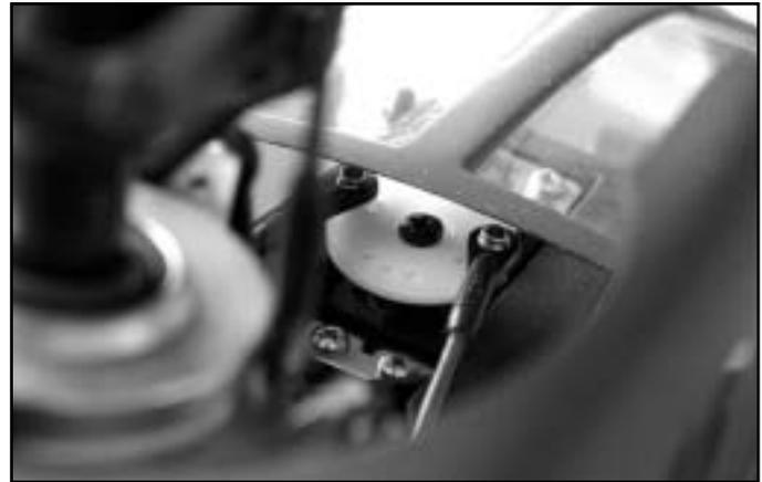
**16.** Trial sit on the landing skid assembly. For Raptor owner, position the Front Windshield in place and check if the ball links on aileron servo horn contacts the front windshield when it is in maximum positive pitch. Lower the Raptor by enlarging the landing strut opening to the fuselage center liner if the servo horn contacts the windshield. It might be necessary to try several times before obtaining a desirable result.
