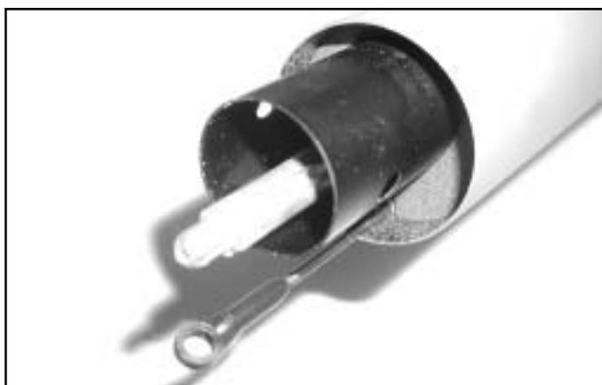
19. Locate a sponge as the Tail Boom Retainer, install the sponge on the tail boom section where the plastic tube for the sponge insertion. Be careful not to apply any glue inside the plastic tube and make sure the pushrod can
