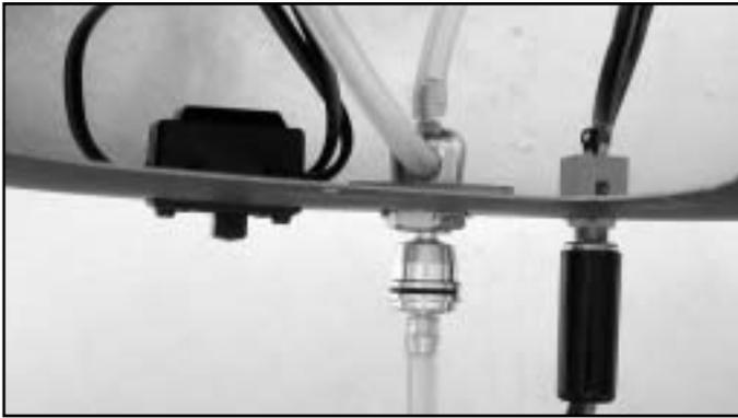
32. You will have to install the remote glow plug adaptor (TTR3803). With the opening for engine cooling located at the bottom of the engine, you can either use the glow starter from the opening or install a Built in Glow Plug Extension Wire (TTR2174) and secure the connector on the fuselage for easy glow ignition. Also suggested is the use of Precision Fueler Valve (TTR1115) which is very convenient for both re-fueling or de-fueling and could filter the fuel when fueling.
