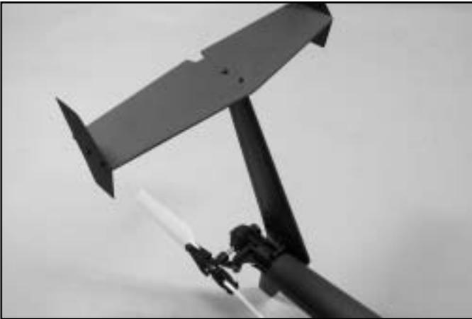
**22.** Trial fit the Horizontal Tail onto the vertical fin, note that flat surface should be facing up and the other side with the air foil facing down. It might be necessary to file/sand the contact area on the vertical fin so that they make perfect contact. Apply epoxy at the contact area and make sure it is perpendicular after securing it with two 3x18mm Wood Screws and two M3 Washers. Secure two vertical Tip Fins onto horizontal tail with four 3x8mm Wood Screws.
