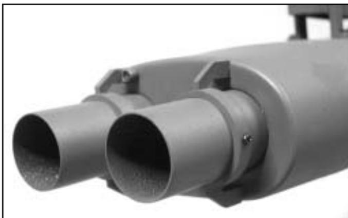
29. Locate the Vents (fiberglass tube) and rings, position the two vents at the tail of missile pod then secure the ring on the tail with four 2x5mm Wood Screws. The vents should stay firmly in the place. Drill 1/16" (1.5mm) holes on the vent then secure the vent firmly with 2x5mm wood screw.
