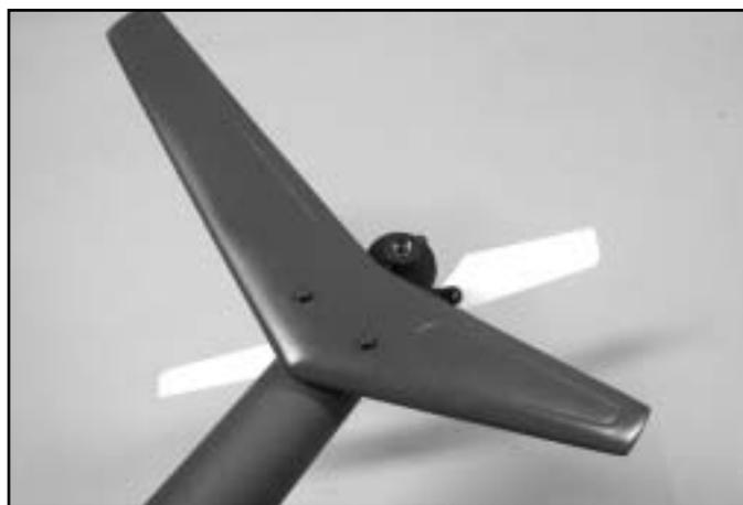
21. Secure the Vertical Fin in place with two 3x40 Socket Screws, two M3 Washers and two M3 Locknuts.
