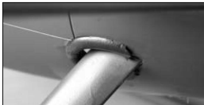
**10.** Locate four Rubber Rings, trim away the flashing and center portion. Place the Rubber Rings at the four landing strut openings. It might be necessary to trim the opening larger to fit the rubber ring with the inserted Aluminum strut. For the rear strut opening, you may cut the ring for easier access.
