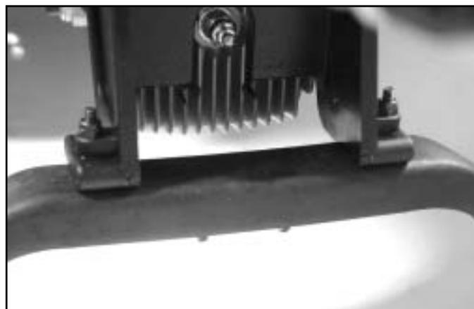
20. Secure the helicopter onto the landing brace with four 3x30mm Socket Screws and M3 Locknuts. Secure the rear brace first then the front.
