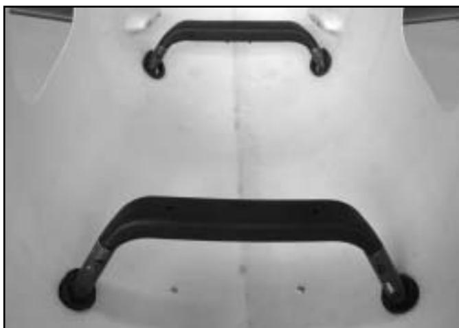
**13.** Remove the landing skid assembly from Heli. Remove the brace from the aluminum strut. Do not remove the strut and skid pipe as they are already adjusted and secured. Apply masking tape on the strut that is going to make contact with the fuselage, since the masking tape will protect the paint from scratching. Place the brace on the fuselage and install the strut and skid pipe onto the brace. You may apply Vaseline on rubber ring to increase the lubrication for easier installation.
