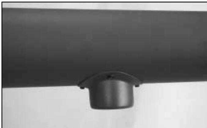
27. Locate the FLIR and place it at the center of the tail section either at the top or bottom. Drill four 1/16" (1.5mm) mounting holes and secure the FLIR with four 2x5mm Wood Screws.
