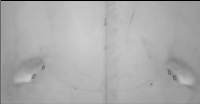
6. Fit the wing in place again, drill two 5/64"(2mm) holes through the wing mount to the wing from the inside of the fuselage. Remove the wing again, apply epoxy at glue area and secured it with two 3x15mm Wood Screws. Either wipe off the excess epoxy or use masking tape to tape the guideline to keep the wing clean after the masking tape removal.
