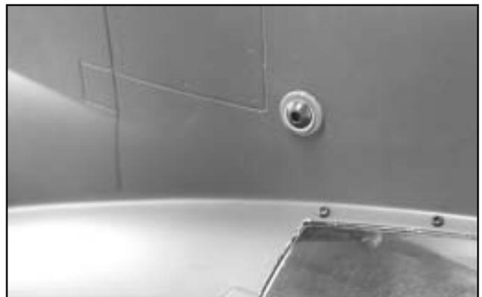
**26.** Secure the fuselage with 4x10mm Button Head Screw and M4 Washer as shown.
