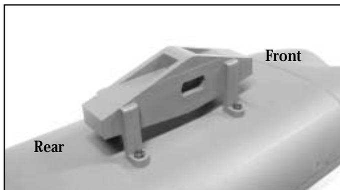
28. Locate the Pod Retainer and center it on the missile pod (the missile pod with square molded line should face down). Drill 1/16" (1.5mm) holes then secure it with 2x8mm Wood Screws. Note the orientation of the retainer.
