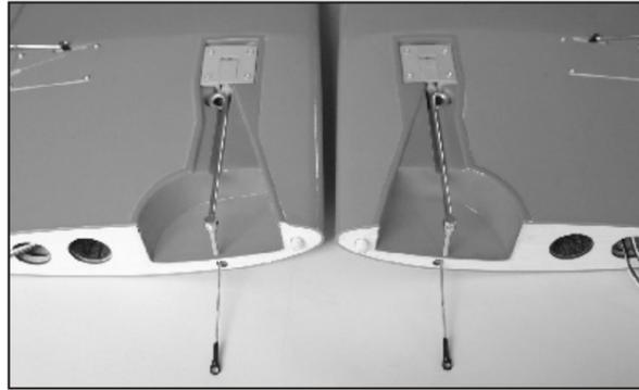
29. You may need to trim the wires of retract so the wheel axle is level to the wing root. Secure the retract in place with four 3x15mm Sink Head Screws. Flats should be ground on the landing gear legs for the setscrew to prevent the wheel axle from rotating under load.
