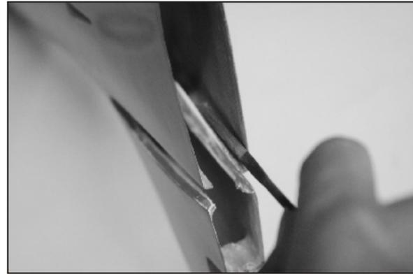
52. Sand the tail saddle to increase the roughness as well as inside of the flange as the fiber cloth will be applied later.
