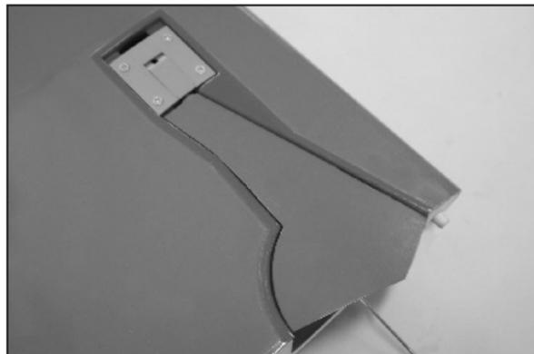
31. Trim the retract door to fit the retract well. 修整輪艙蓋並確認與輪艙搭配完美。
