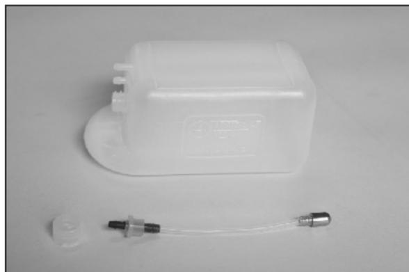
Locate the fuel tank and its accessories. Assemble the tank as shown. Install the fuel tank in place, connect the fuel lines and exit from the firewall for enough length to carb and muffler.
