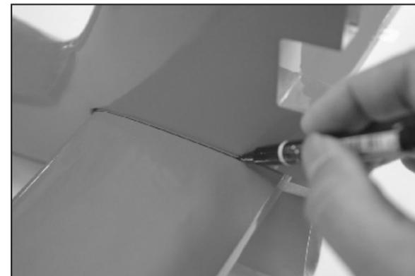
48. Trial fit horizontal tail in fuselage, center it then make marks on tail at four sides.
