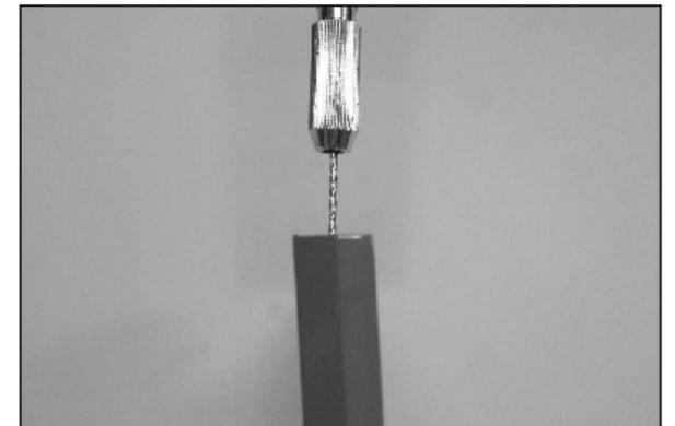
17. Carefully drilling the joiner side at mark. Note that it is angle at the joiner side please drill the hole perpendicular to the surface. Drill 2.5mm hole on Flap I and 2mm hole on Flap II.
