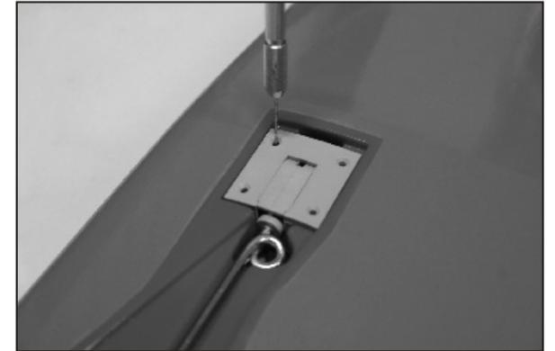
26. Place the retract in place and drill 5/64" (2mm) holes on the retract mount.
