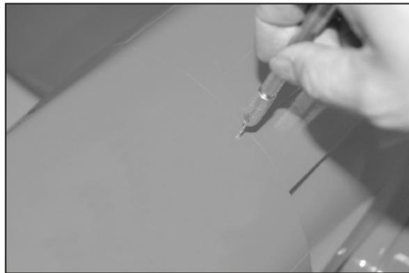
87. Install the engine cowling; first glue the plywood doublers inside the fuselage at where hole is. Trial fit the cowling in place and temporarily secure it with mask tape. Drill 1/16"(1.5mm) at the place where doublers are.
