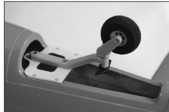
71. Secure the tail gear assembly on the tail gear mount with 4x20mm sink machine screws.
