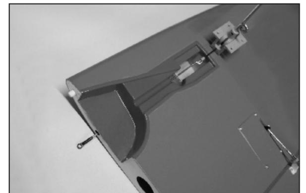
28. Insert the pushrod from wing root then connect to retract. Note: The ball end with "Tiger" side should face upside of wing.
