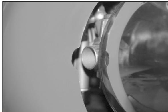
90. Suggest to file the cowl located near the vent of carburetor as shown, the engine will get enough air and run smoother if you install a 2 stroke engine.
