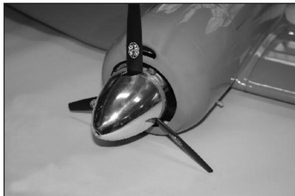
89. Install the propeller and furnished spinner. What we used here is Master Airscrew 13x8.
