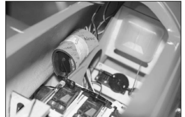
85. Connect all servo wires to the receiver; wrap the receiver with foam to fully protect the receiver. Insert receiver between frame and fiberglass wall in fuselage. 連接伺服機線至接收機。將接收機裹以泡棉保護。將接收機置於機身與側板之間。
