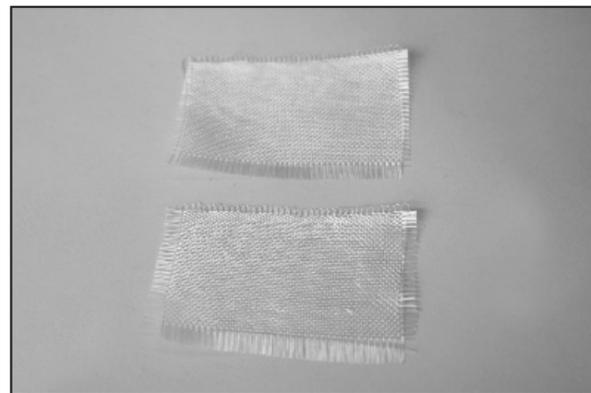
54. Locate the fiber cloth then cut into two pieces at about 100 x 80mm (4 " x 3").
