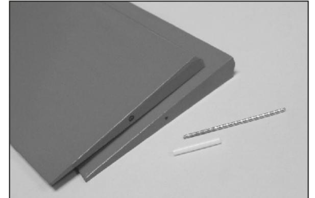
16. Locate the joiner wire and guide tube. Make mark at the center of the joiner side of the Flap I and Flap II. 設置連動鋼絲以及導管。在內、外側襟翼的中間做記號。
