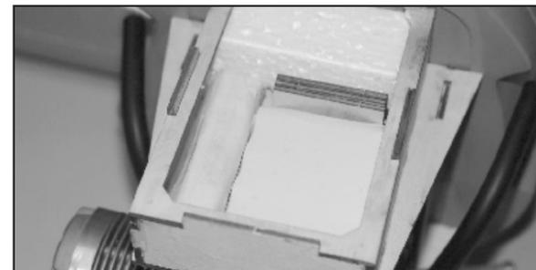
83. Place a battery in the battery case; use double side tape to secure it in the front of battery case. You can use the excess servo tray plywood to make a block to hold battery in place. It requires an extension wire to connect to the switch harness. Approximately 300-350g of weight will be added in the front of the battery case. See balance section in page 24 and add proper weights to get right CG. 使用1000mAh 以上電池 固定於電池盒中 連接延長線接至開關。電池盒請再加重約300-350g 注意電池盒後方以發泡固定之。重心位置請參考末頁平衡一節。
