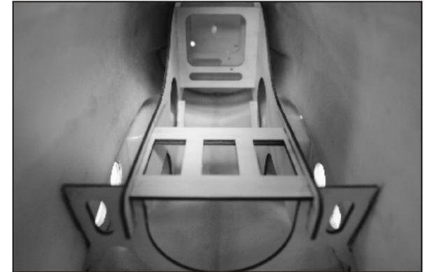
38. The side frame is either marked L or R. Make sure L is at left side and R is at right side. Always trial fit all wood parts before you glue it. Suggest to glue the one side frame in place first, next the other side frame with servo tray at the same time. Fuel tank retainer and retract servo mount strips at the last.
