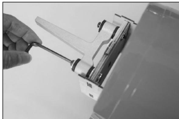
45. Install the Anti-Vibration Engine Mount in place with 5x40mm Socket Cap Screw and Blind Nut. You just screw in the cap screw then the blind nut will punch into the firewall.
