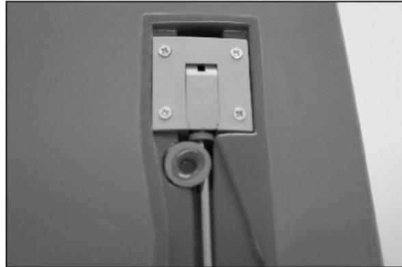
32. Sand the upper retainer B and place it in the strut coil then apply CA on retainer. Next place the wheel door in place, the retainer will be glued on wheel door precisely. 在腳架收起的狀態下將輪艙蓋固定件B置於緩衝環上，使用瞬間接著劑於固定件B，然後將輪艙蓋置於其上使其固定於輪艙蓋。
