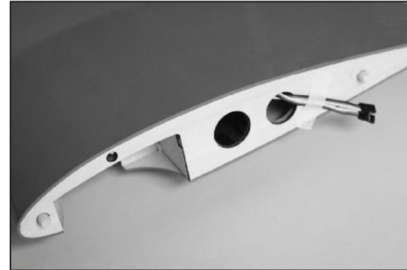
23. Epoxy the dowels at wing root in place as shown.
