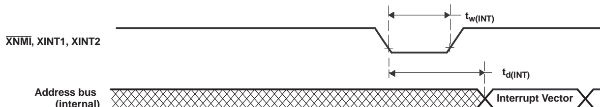
Figure 6-17. External Interrupt Timing
