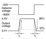
The tr time period defined as the time required for the output voltage to rise from 10 to 90% in response to a 1ms min. step decrease in measured voltage from -20 to -900V.
