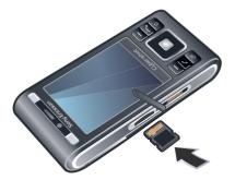
Open the cover and insert the memory card with the gold-coloured contacts facing up.
