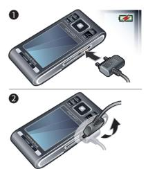
1 Connect the charger to the phone. It takes approximately 2.5 hours to fully charge the battery. Press a key to view the screen.
