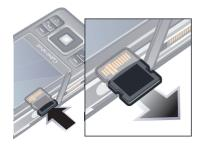
Open the cover and press the edge of the memory card to release and remove it.
