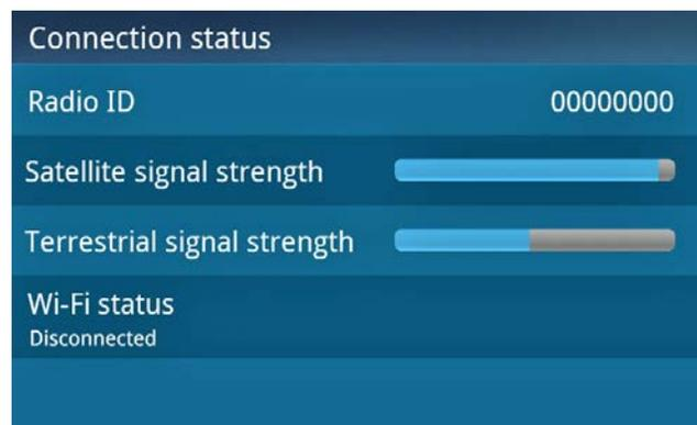
While observing the signal strength, make small adjustments to the angle of tilt of the clamshell until the highest possible signal strength is achieved. Also turn the antenna slightly to the right or left and observe if the signal strength increases. For each tweak, allow a few seconds in each position to determine if the signal strength increases.
