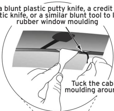
Tuck the cable under the moulding around the window
