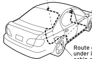
Route cable from trunk under interior trim, into cabin and towards front of vehicle
