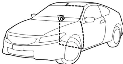
of the door opening and route it under the carpet toward the dashboard. Coil any excess cable in a hidden location, such as under the carpet, keeping it away from any vehicle pedals or controls. Secure the excess cable with wire ties.
