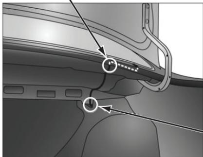
Route cable along trunk wall and into cabin through gap or conduit, along existing wiring harness
