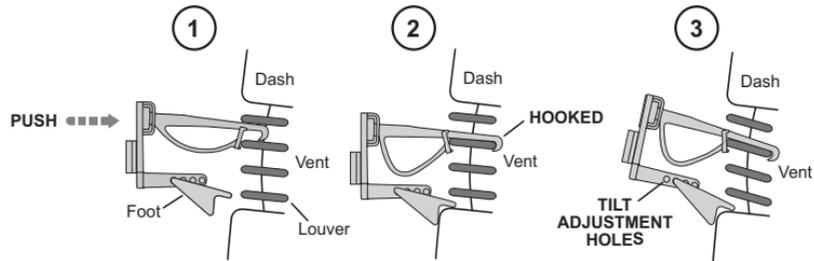
To remove the Vent Mount, push the mount into the vent. Then lift up until disengaged from the rear of the vent louver, and remove the Vent Mount.
