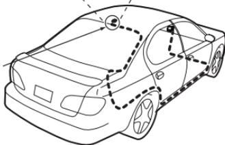
Route cable out from under rear windshield moulding and tuck into weatherstripping around trunk opening
