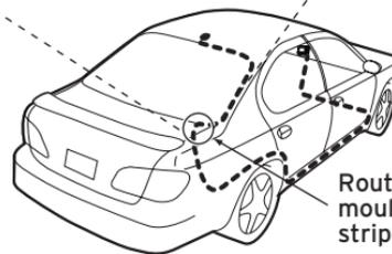
Route cable out of window moulding and into weatherstripping around trunk opening
