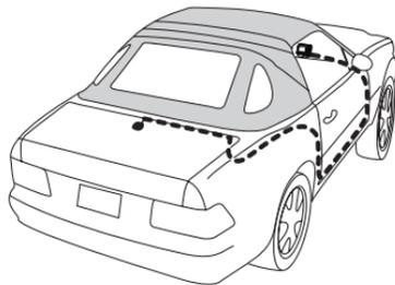
underneath. Avoid side airbag locations on back pillars and above the doors. Airbag locations are marked with "SRS" logos. Be careful not to crimp or cut the cable.
