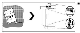
Level the Appliance Adjust the height of the front feet of the refrigerator, and ensure an upright and stable placement.
