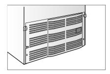
The ventilation grid on the compressor cover at the back of the refrigerator must not be covered or blocked. Avoid placing the refrigerator close to a heat source or subjecting it to direct sunlight.
