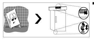
Level the Appliance Adjust the height of the front feet of the refrigerator, and ensure an upright and stable placement.
