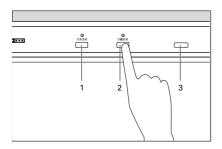
Buttons 1 and 2 on the fascia are used to turn on or turn off the freezer and refrigerator compartments, respectively. The user can turn on or turn off either of two compartments as needed.
