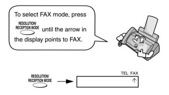
When the reception mode is set to FAX, the fax machine will automatically answer all calls on four rings and receive incoming faxes.
