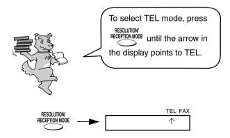
When the reception mode is set to TEL, you must answer all calls by picking up the fax machine's handset or an extension phone connected to the same line.
