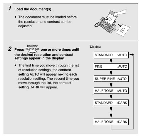
**Note:** In order to transmit in SUPER FINE resolution, the receiving fax machine must also have that resolution. If it doesn't, your machine will automatically step down to the next best available setting.
