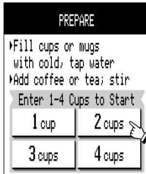
2 Touch desired number on the screen. The oven will start automatically.
