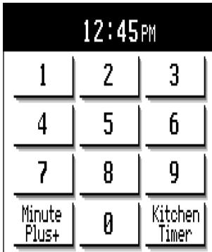
The Home Page is the beginning. It shows the time of day, if the clock has been set. It also shows Minute Plus +, where by touching the screen the next screen appears, making it easy to select one of twelve commonly used times. Touching Kitchen Timer tells the oven that the time set is only for timing, not for cooking.
