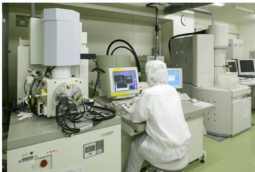
Conducting analysis using FIB
