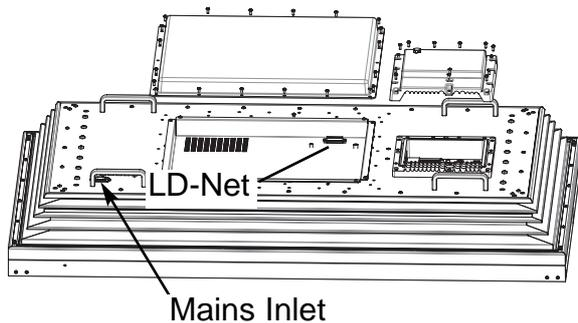
1. Connect the in-line power connector to the Mains Inlet as shown above.
