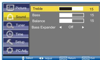
Select and adjust to obtain the best sound settings for your environment using the **PA** or **PV** button to select **Treble**, **Bass** or **Balance** and the **▲**+ or **▲**- button to adjust levels.
