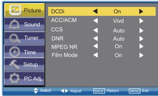
**DCDi**(Directional Correlational Deinterlacing) is used to process moving angled edge in deinterlacing to get the smoothest and most natural image. Press the **▲**+ or **▲**- button on the remote control to select **On** or **Off**.
