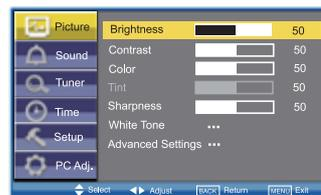
2. Use the **▶** or **◀** button to select eg. Brightness and the **▲+ or ▼-** button to adjust levels.
