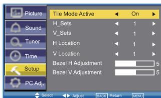
**H\_Sets** is used to divide the horizontal picture into more than one part, but the most is 5 parts (5 monitors).
