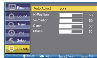
**Auto Adjust** is used to automatically detect incoming signal, and adjust itself to optimize its performance by using the **▲+** or **▲-** button. If the image is not displayed properly, a manual adjustment is required (Refer to following adjustments).
