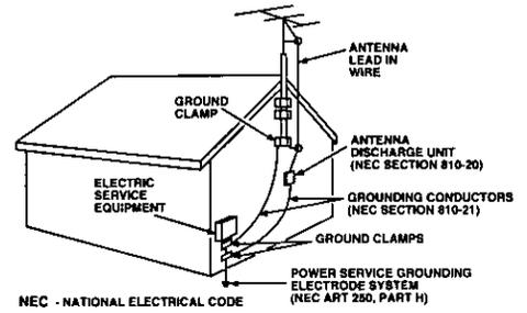
information with respect to proper grounding of the mast and supporting structure, grounding of the lead-in wire to an antenna discharge unit, size of grounding conductors, location of antenna discharge unit, connection to grounding electrodes and requirements for the grounding electrode.
