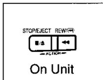
You can operate the menu screen using the unit buttons. To display the menu, press STOP/EJECT and REW/FF together with no tape inserted. To exit the menu, repeat above with or without tape inserted until normal screen appears.
