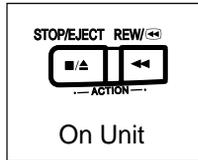
You can operate the menu screen using unit buttons. To display the menu, press STOP/EJECT and REW together with no tape inserted. To exit the menu, repeat above with or without tape inserted until normal screen appears.
