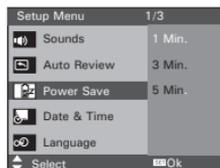
**1/3/5 MIN** The camera is designed to switch off automatically to save battery life after the specified period of inactivity.
