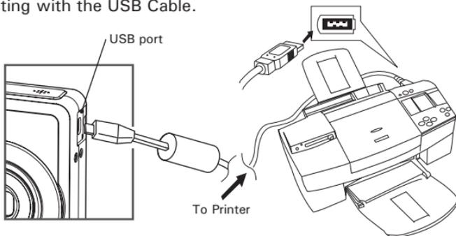
1. Plug the labelled end
