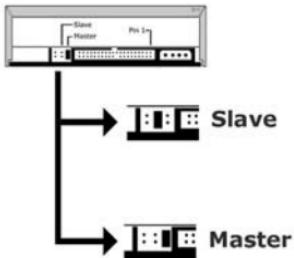
**EN** If you replace a drive, take it out and check which setting it has ("Master" or "Slave"). Remember this setting and go to step 10.
