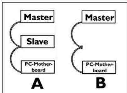
**EN** Connect the IDE cable like in A (2 devices) or B (only 1 device).
